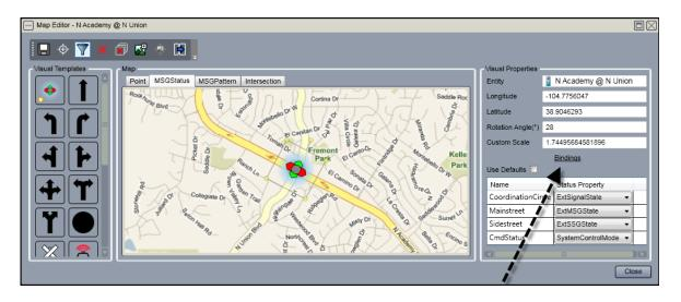
4 For each icon that represents an element that can change state (for example, a phase, a detector, a railroad preempt, etc.), you must associate the icon with the appropriate state property. To do this, use the Bindings section of the window.
