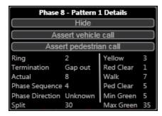
To put a temporary call on a phase, click **Assert vehicle call** or **Assert pedestrian call**. Click the button again to turn off the call. (When you close the Signal Status display, Centracs asks whether you want to remove the call.)
