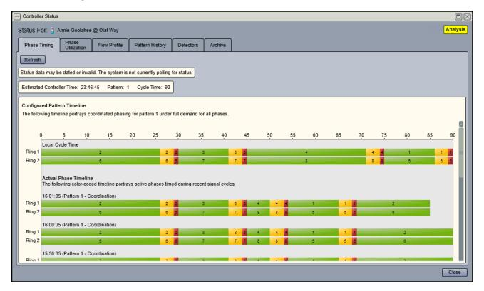
The Configured Pattern Timeline shows the programmed splits. The numbers shown inside the colored bars are the phase numbers. The Actual Phase Timeline shows the actual splits for the last 15 minutes. A black bar indicates no data during that time (for example, when an upload is in progress, no polling is done).
