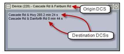
This window shows a list of the destination Data Collection Stations with which this DCS is paired as the origin, and shows the current travel time for each link pair. The example above shows two link pairs: in both cases, "Device (220) - Cascade Rd & Fairburn Rd" is the origin DCS, indicating the direction of travel for these link pairs. For more information about origins and destinations, refer to *Overview of Travel Time* on page 14-2.
