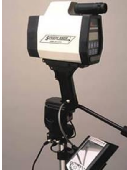
Figure 33. The SpeedLaser® Model of Laser Speed Gun (Source: http://www.laseratlanta.com )
