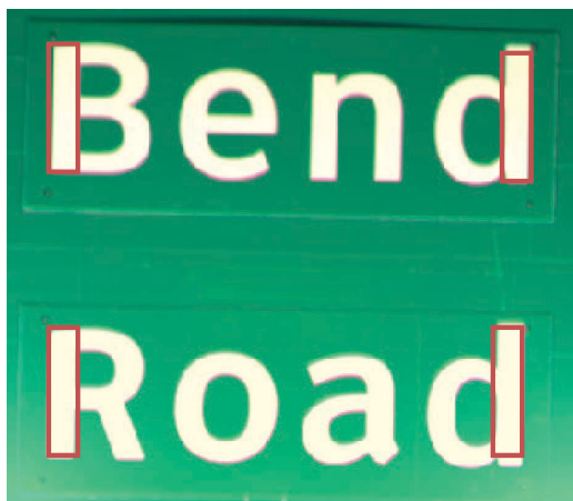
Figure A-1. Sample areas for calculating averaging luminance.
