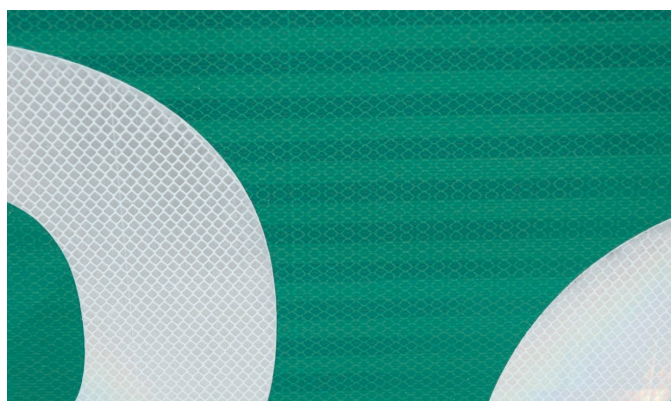
Figure 7. Type XI prismatic legend on Type IV prismatic background.
