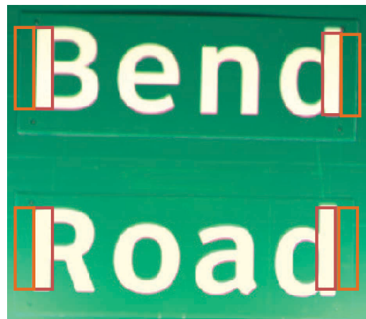
Figure 9. Rectangles selected for calculating sign luminance and Weber contrast.
