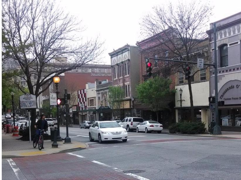
*Figure 7 While pedestrian signal heads may not be required at a typical urban signalized intersection, pedestrian signal heads and marked crosswalks may make sense to provide consistency in application throughout a downtown system.*
