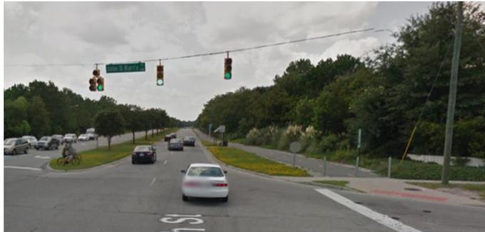
*Figure 6 Protective-permissive left turn signals may be confusing to pedestrians attempting to rely on the vehicular traffic signals to know when it is their turn to cross, and therefore engineering judgement must determine whether Section 1.3.2.1 D of the 2009 MUTCD applies.*
