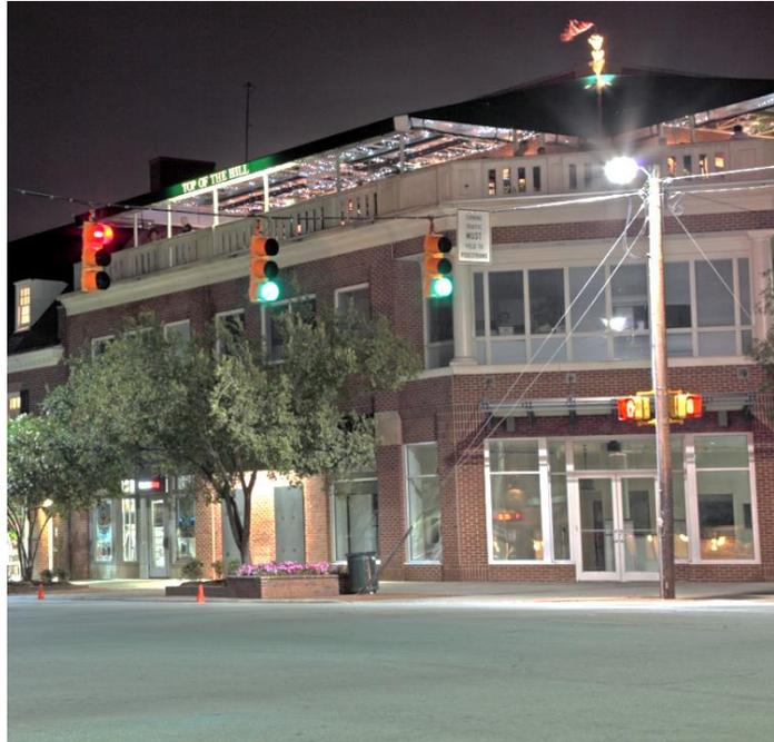
Figure 15 Depending on pedestrian and traffic volumes, a traffic signal may be warranted. If Warrant 4 or 5 of the MUTCD are met, and the traffic signal is installed, then pedestrian signal heads are also required. Photo credit: Caroline Culler, Wikimedia Commons
