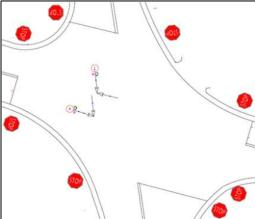
Example crash diagrams from a spot safety project evaluation. The countermeasure involved converting an intersection from two-way stop control to all-way stop control in Wake County, resulting in a 75% reduction in crashes.
