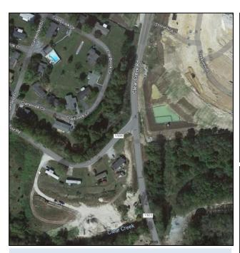
Example VEWF Site with sight distance factors such as an embankment and vegetation, as well as curvature and intersection skew. This site demonstrated a reduction in total crashes comparing 3-year before and after periods.
