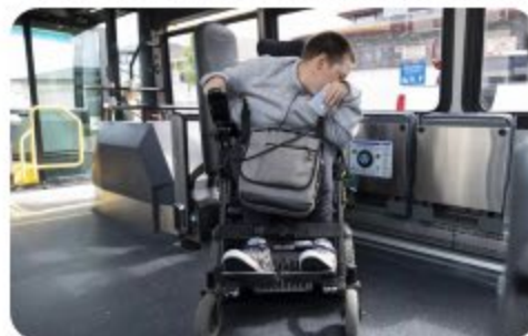
Q'Straint Quantum autonomous wheelchair securement system
