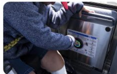
Q'Straint Quantum autonomous wheelchair securement system
