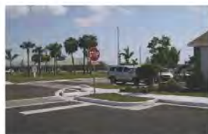
Bulb-outs at intersections (Improved visibility)
