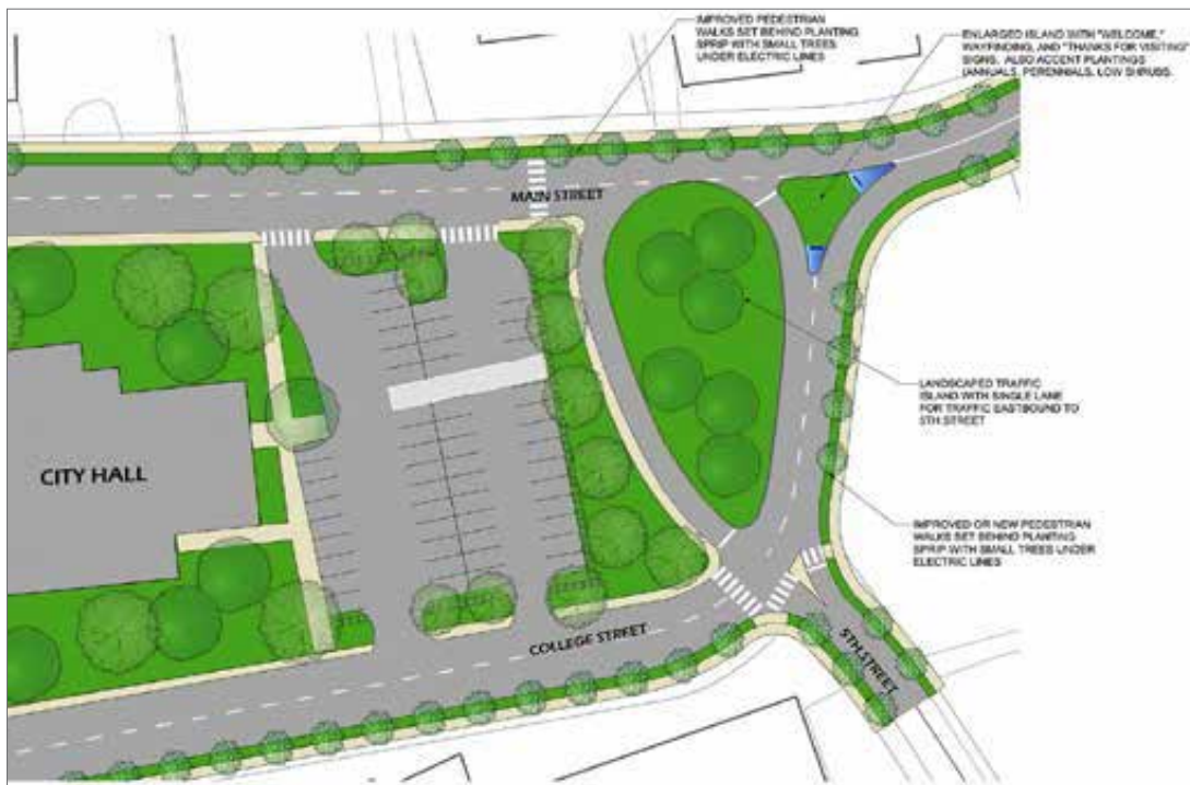
The figure above depicts a concept plan for realigning the intersection of Main Ave. and College Ave. to improve vehicular circulation and pedestrian safety. (Source: Newton Streetscape Master Plan & North Newton Master Plan)
