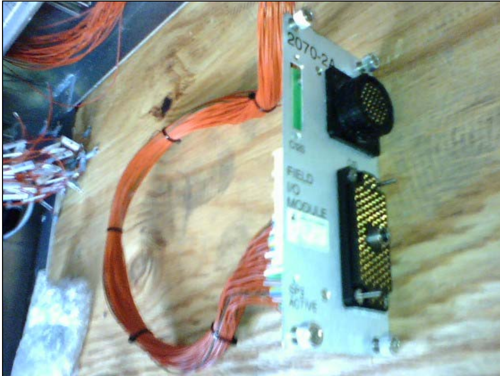
Figure 4.16 170 Cable with a C1 Back Panel on One End and Individual Wires on the Other
