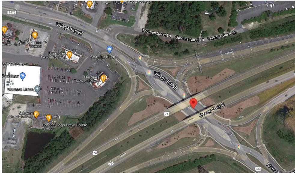
Figure 10-2: Aerial View of the Diverging Diamond Interchange on US-17 (and US-74 and US-76) at Village Road / River Road in Leland, NC
