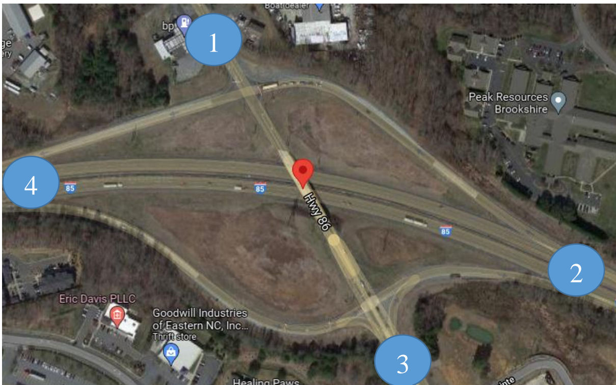
Figure 8-1: Plan View of Traditional Diamond Interchange at I-85 and NC 86 with Indicated Origin and Destination Labels
