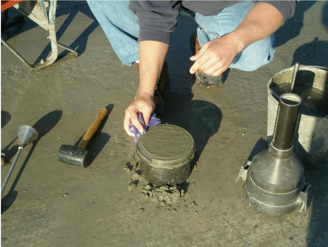
Clean the rim of any concrete residue.
