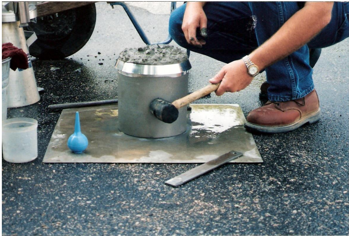
Tap the sides 10 – 15 times to consolidate.
