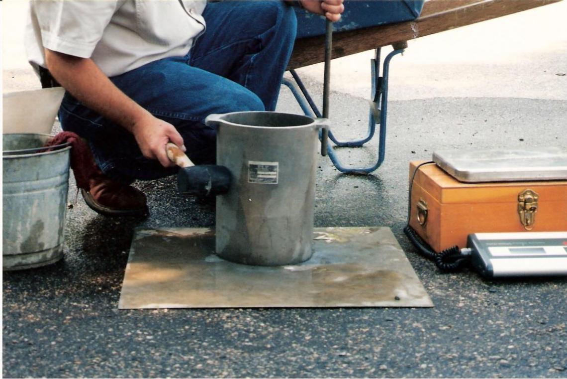
Consolidate the concrete by tapping the sides of the bucket 10 – 15 times.
