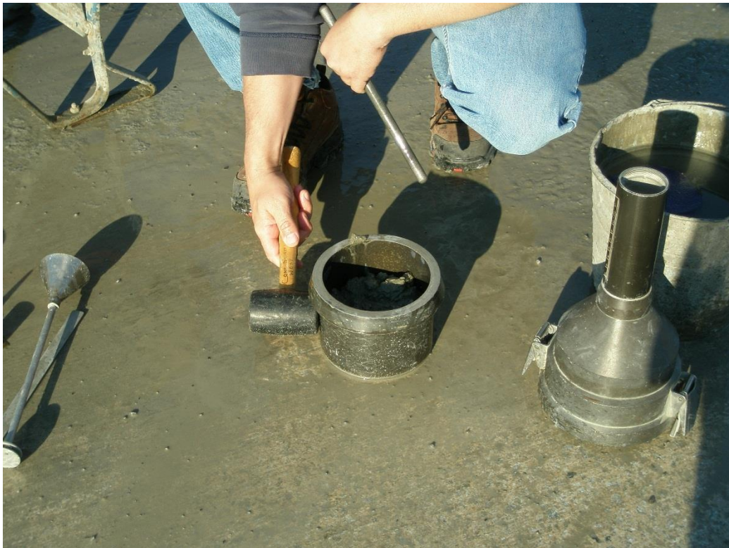
Tap the sides of the bowl 10-15 times to consolidate the concrete.
