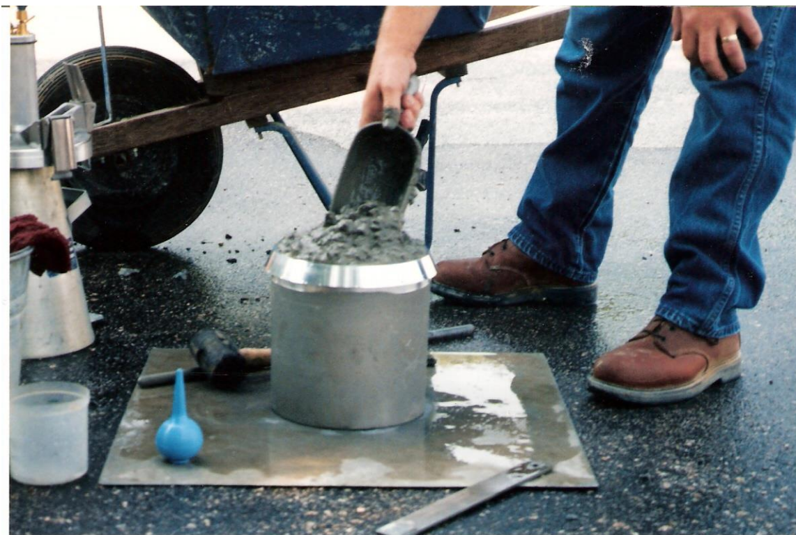
Fill the third and final layer (slightly overfill).
