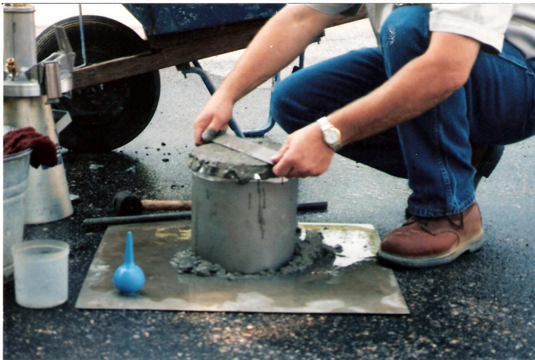
Remove all excess concrete with the strike-off bar, creating a smooth finish.
