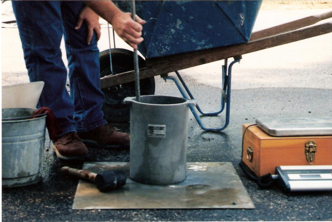
Rod the second layer, penetrating the first layer by 1 in.
