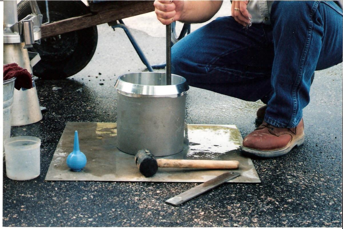
Rod the second layer 25 times, penetrating the first layer by 1 in.
