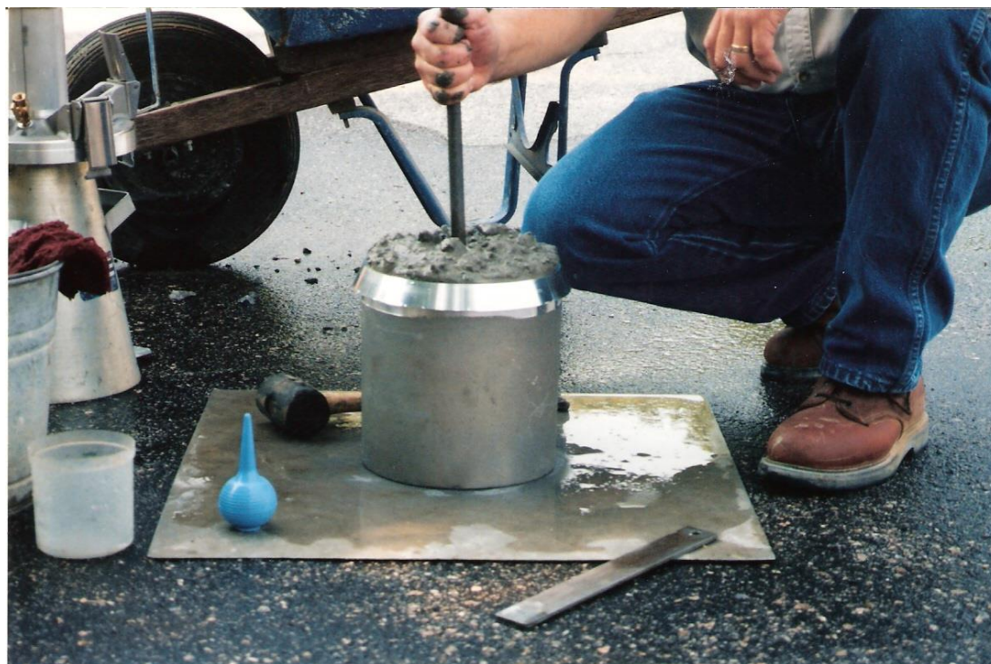
Rod 25 times, the rod penetrating 1 in. into the second layer. Distribute the strokes evenly.
