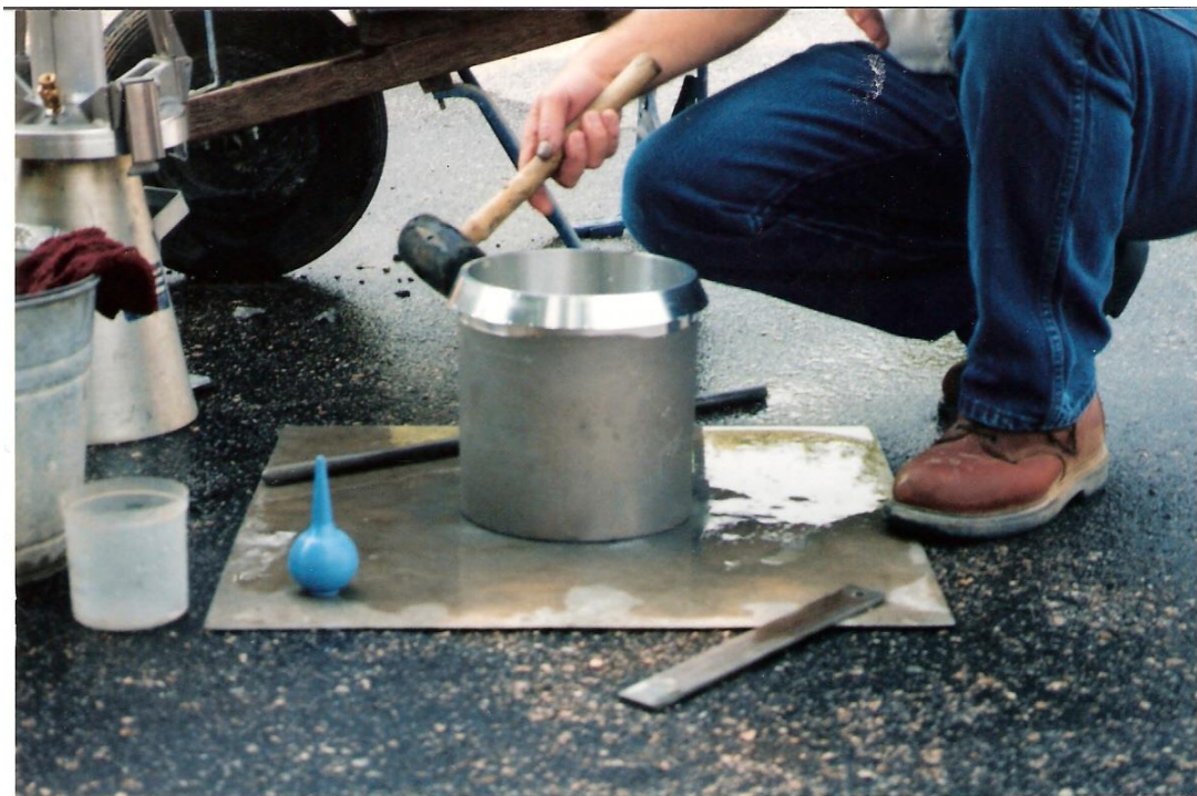
Consolidate the second layer by tapping the sides of the bowl 10 – 15 times.
