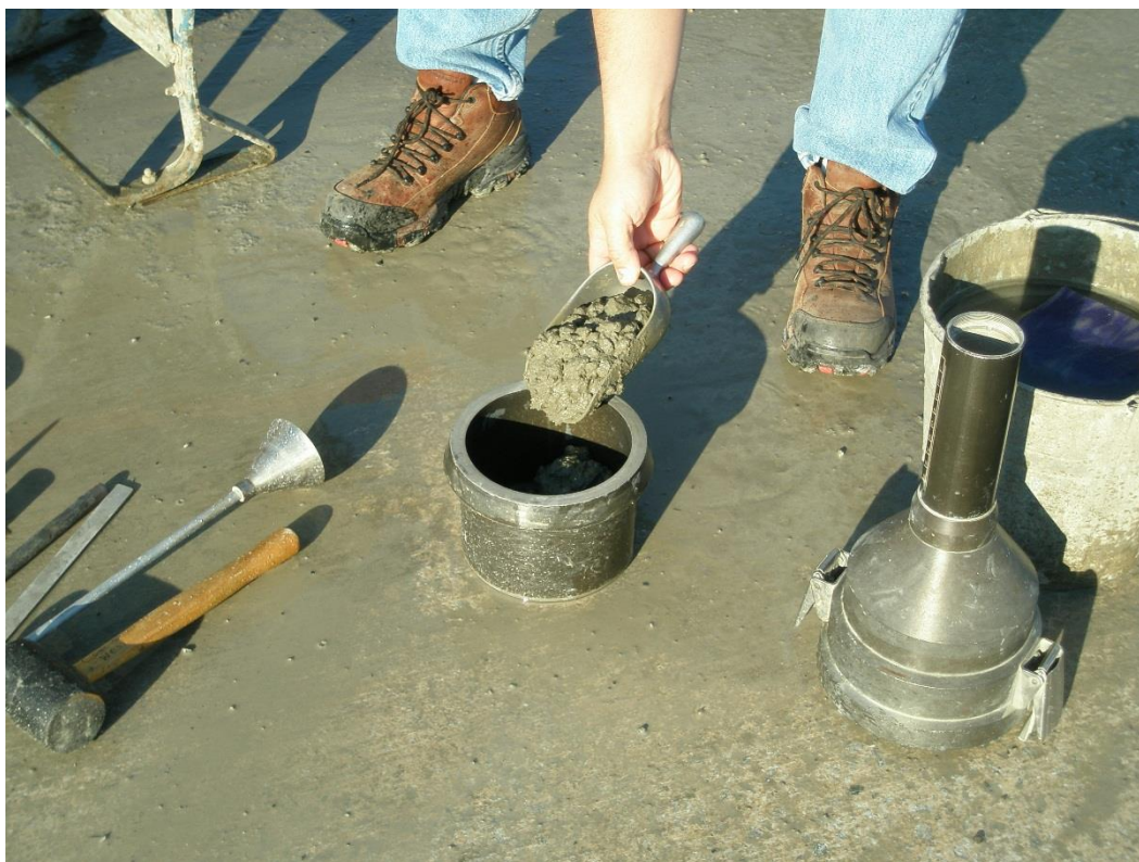
Fill the 1 st layer with concrete to about half of the volume of the bowl.
