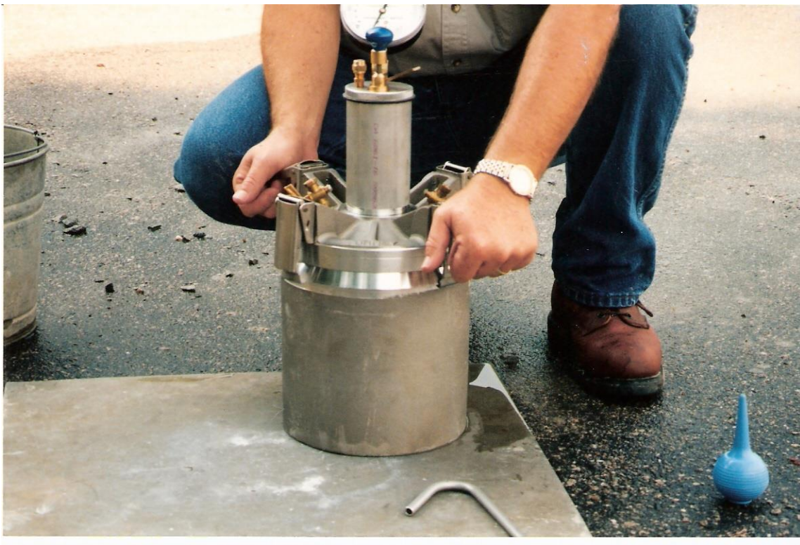
Securely clamp the lid onto the base. Alternate side clamps should be tightening simultaneously.
