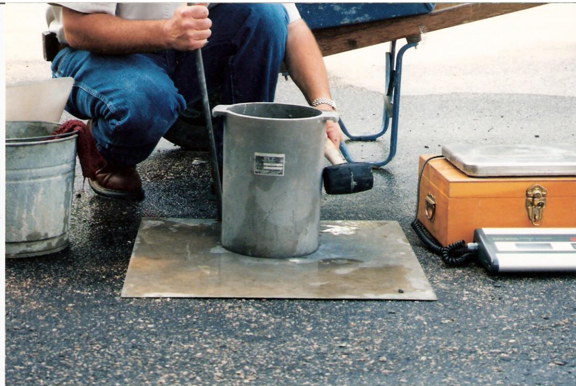
Consolidate second layer by tapping side of bucket 10 – 15 times.
