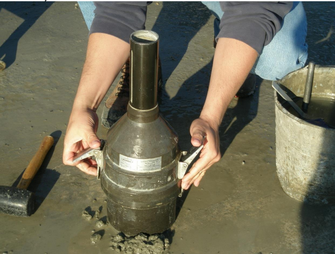
Moisten and clean the lid gasket. Clamp top to the base.
