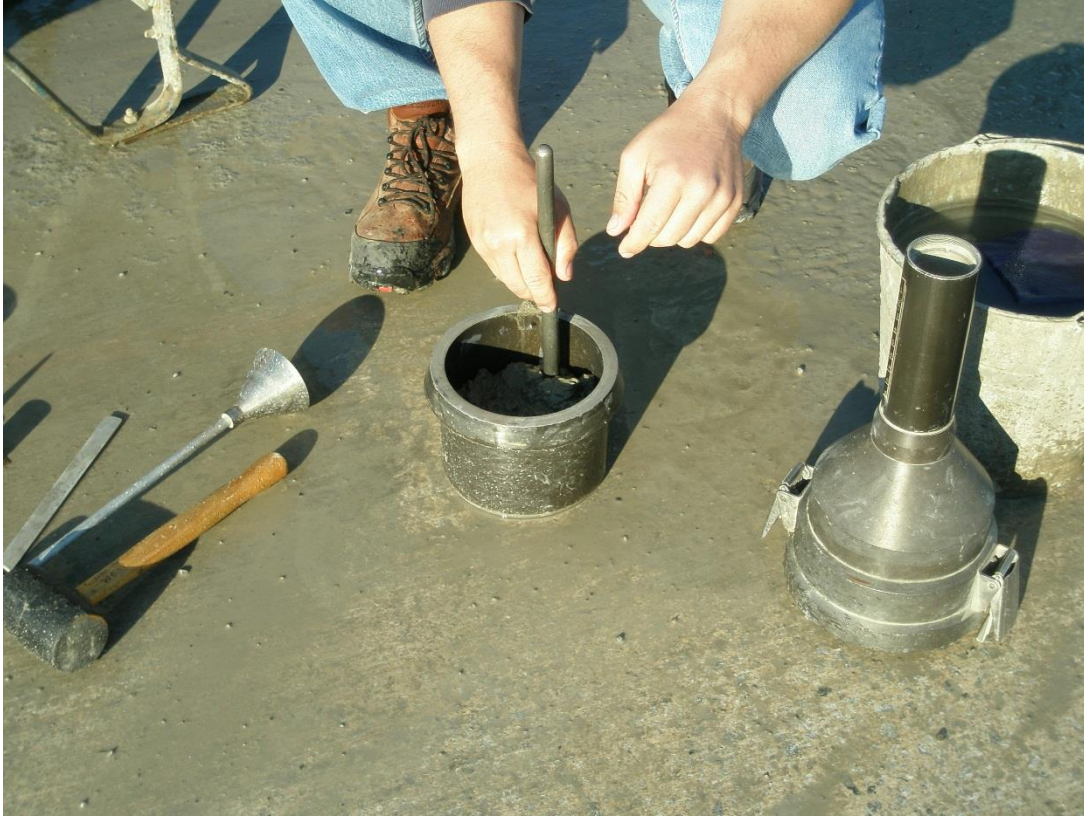
Rod the first layer 25 strokes
