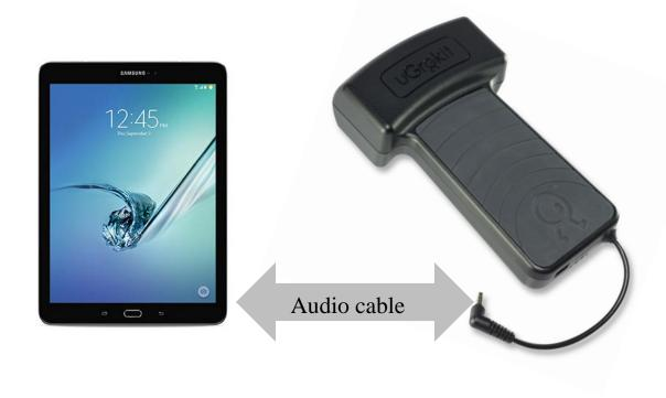
• Connect the Grokker Scanner to the tablet by plugging the Grokker audio cable into the tablets audio port.
