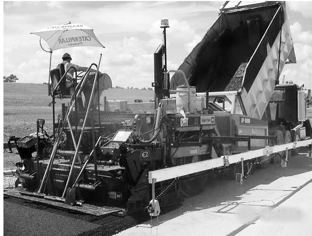
Figure 9-9 Long Mobile Grade Reference System (Sonic Type with Referencing Sensors)
