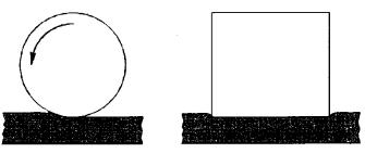
(b) MATERIAL COMPACTED BY ROLLER WITHOUT HORIZONTAL DISPLACEMENT OF MIX.
