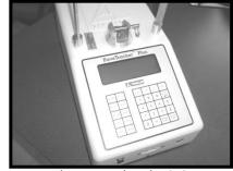
Troxler Pavetracker Plus 2701-B (Density Acceptance for Surface Only)
