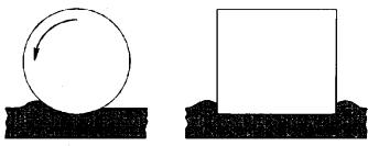
(a) RIDGES AND WAVES CAUSED BY HORIZONTAL DISPLACEMENT OF MIX DURING ROLLING.
