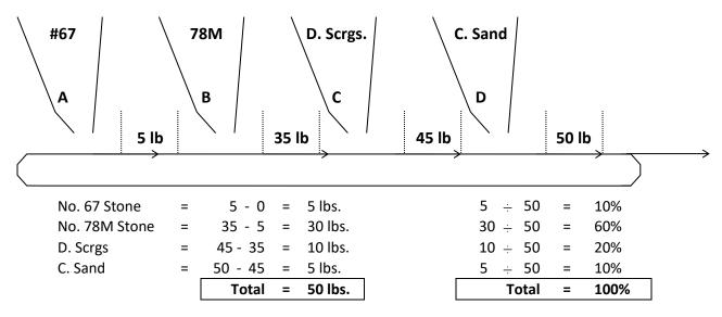
Note: Sample across the entire cross-section of belt for a minimum of two (2) feet. Each section removed after each feeder must be the same length for all feeders.
