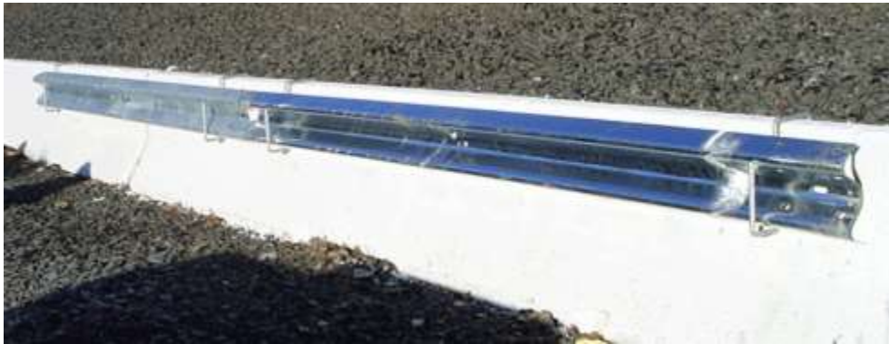
Figure 8 – Section of guardrail on the left shows the effects of wet storage stain, while the right side is unaffected.
