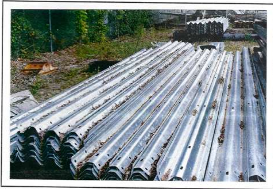
Photo 80 Improper Storage. Decaying matter is in contact with galvanized materials.
