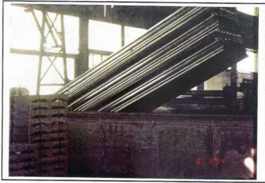
Photo 9 Guardrail leaving the zinc bath. The rail is withdrawn at an angle to help prevent spiked and excess zinc buildup.
