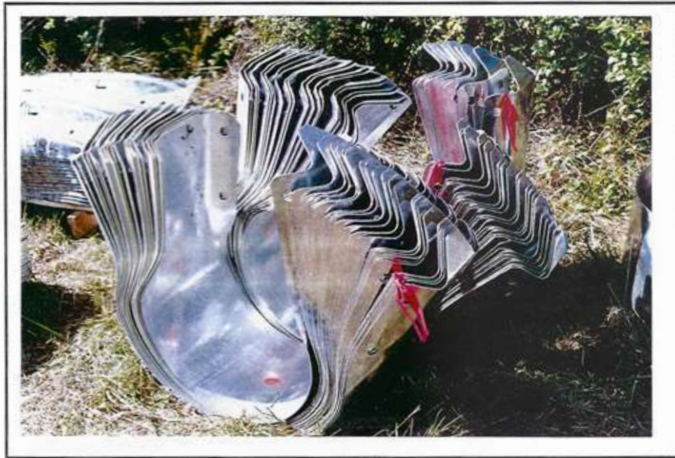
Photo 86 Improper storage. Material should not be in contact with the ground surface or decaying matter. Also, this particular orientation prevents drainage of the pieces, allowing water to collect in the items.
