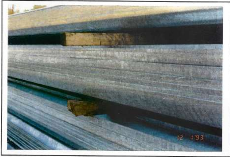
Photo 26 Condition: Dull Gray Coating or Mottled Appearance
