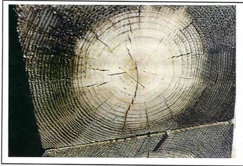
Photo 70 Wood guardrail post. Post should have stamps on both ends indicating that it has been inspected and accepted by NCDOT Consultant Inspectors. Wood post without stamps on both ends should not be used.
