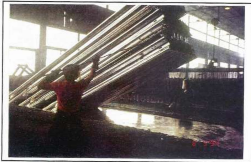
Photo 10 Worker removing excess zinc from the guardrail. This will help prevent spikes and lumps on the rail.
