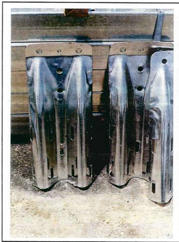
Photo 90 Example of clean guardrail material after galvanizing.
