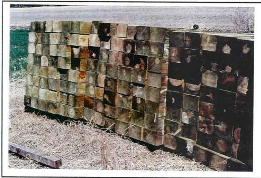
Photo 77 Properly stored and identified wood posts. Each bundle of wood posts should have at least three tags located on the bundle in addition to a stamp on each end of every post.
