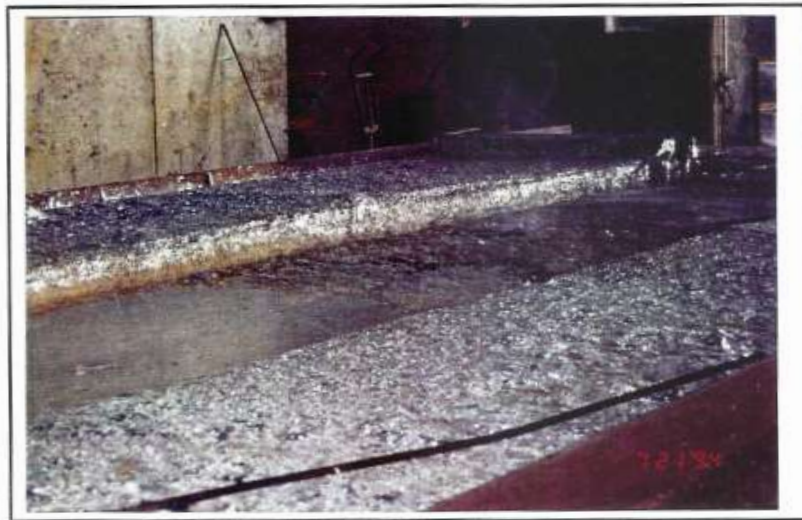
Photo 12 Ash which has reformed after removal of material from the zinc bath. This must be removed before another item is dipped into the tank.
