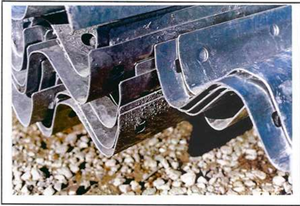
Photo 53 Condition: Ash Inclusion
