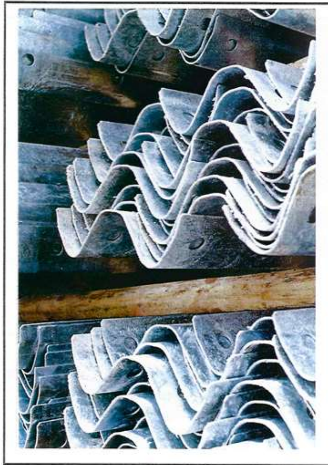
Photo 73 Condition: Wet Storage Stains (White Rust)
