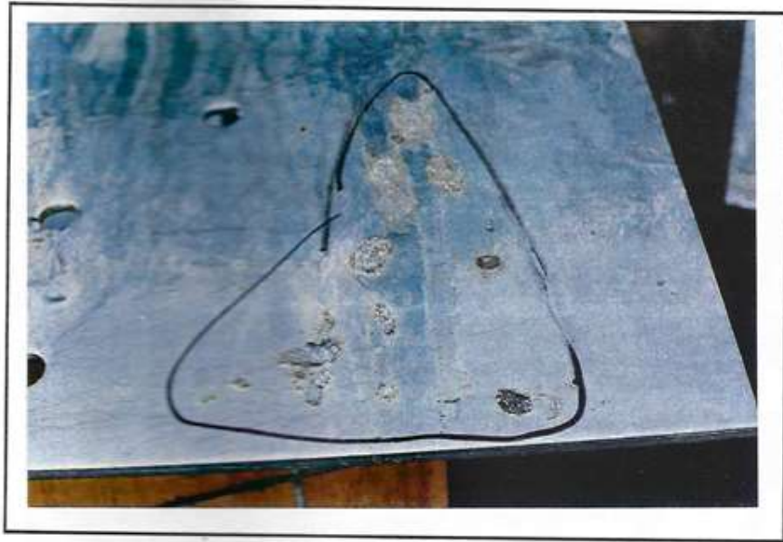
Photo 49 Condition: Ash and Flux Inclusions
