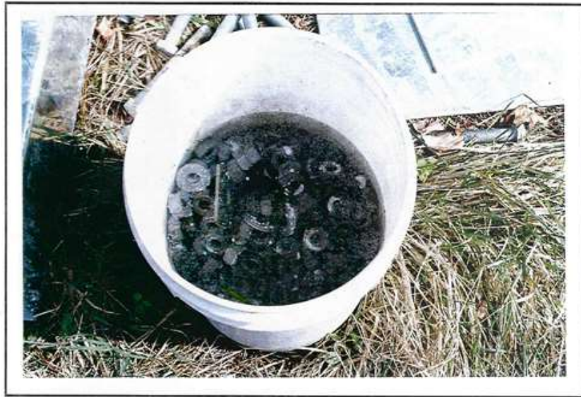
Photo 84 Improper storage of hardware. These materials are rejectable.
