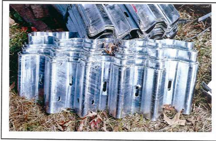
Photo 68 Condition: Excess holes in backup plates.
