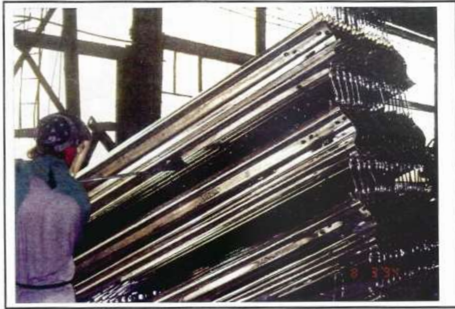
Photo 11 Workers removing excess zinc from the guardrail. This will help prevent spikes and lumps on the rail.
