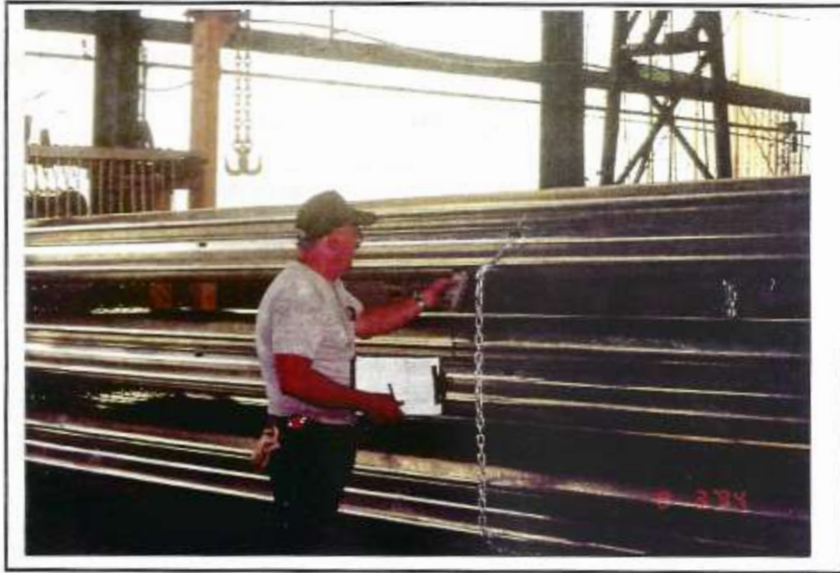
Photo 13 Plant inspector checking the coating thickness.
