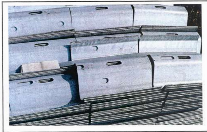
Photo 69 Condition: Excess holes in backup plate
