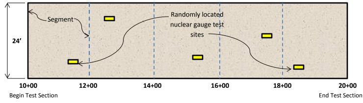
Figure 3 Plan view of test section (not drawn to scale)
