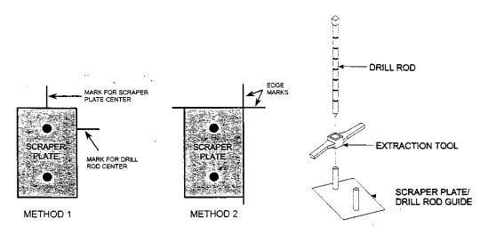
Figure 1 Scraper Plate, Drill Rod, and Extraction Tool (Troxler Nuclear Gauge Operation Manual)
