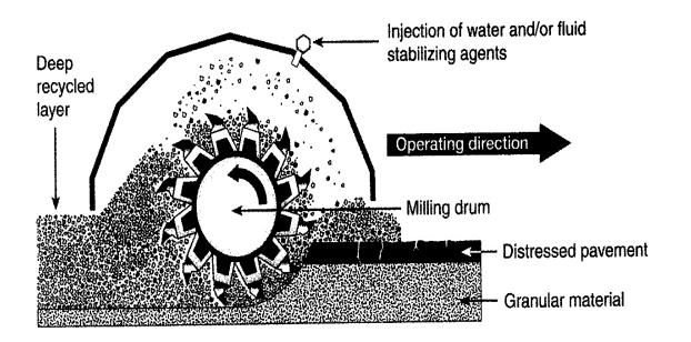
Figure 2 Diagram of Cutting Drum performing FDR (A.R.R.A Basic Asphalt Recycling Manual FHWA)
