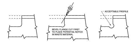
Figure C-3.2—Examples of Good Practice for Cutting Copes
