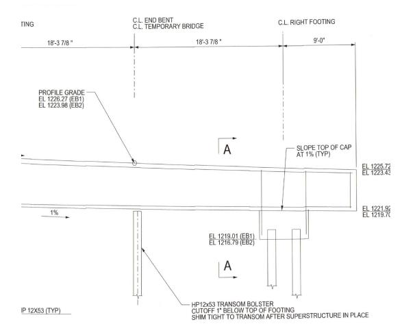
This is an alternative substructure detail that does not show how the bolster is to be attached to the pile.
