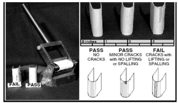
Figure A: TSC Bend Test: Passing and Failing Sample
