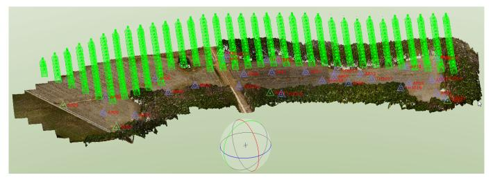
FIG.1: R-2582A ROBINSON 2 PIT - ORIGINAL FLIGHT DENSE POINT CLOUD, CONTROL POINTS, CHECK POINTS, & NADIR FLIGHT LINES
