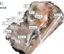
Basins and sediment fence (SF) outlets were located and watersheds determined.
