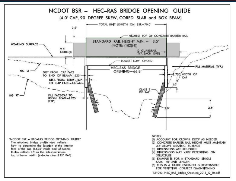
Figure 4. HEC-RAS Bridge Opening Guide (4.0' Cap)
