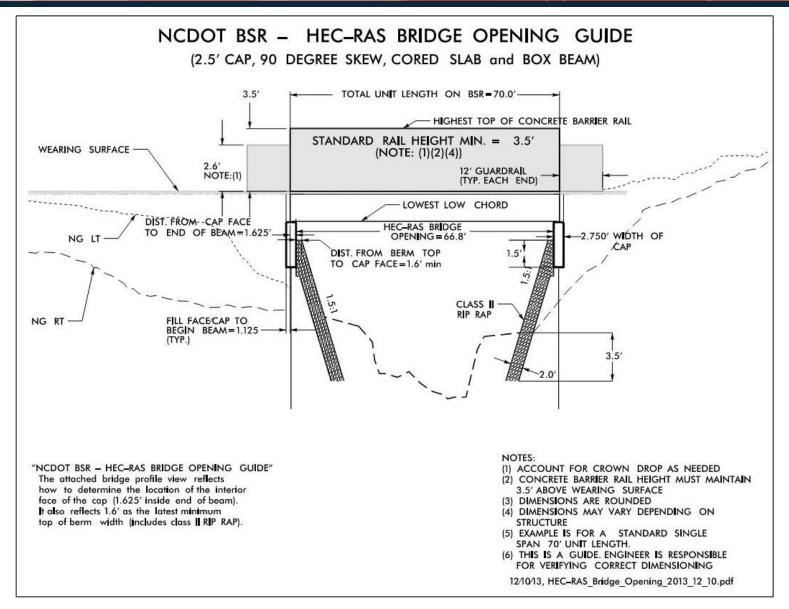
Figure 3. HEC-RAS Bridge Opening Guide (2.5' Cap)
