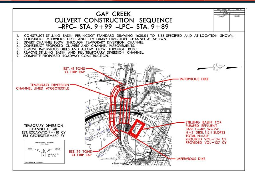
Figure 2. Culvert Construction Sequence Plan Example
