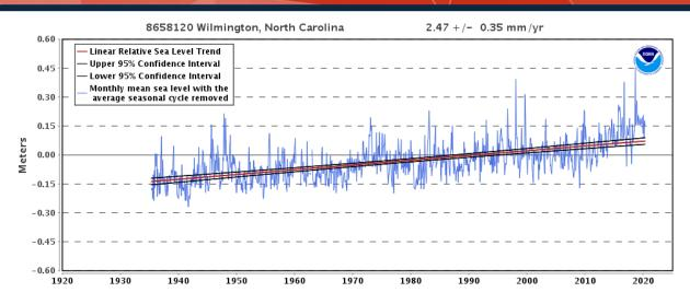
Figure 2. NOAA Gauge Plot of Monthly MSL Data for Wilmington, NC from 1935 to 2019 Showing Relative Sea Level Trend of 2.47 mm/yr. (NOAA n.d.)
