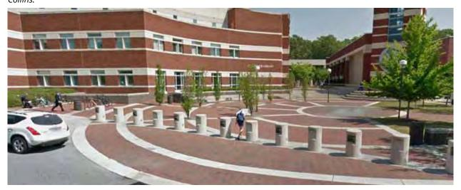
This drop off area in Greenville, North Carolina uses concrete bollards to define the edge of the roadway, but circular patterns of brick pavers and concrete bands visually connect the roadway with the pedestrian plaza. Image courtesy James Sipes.
