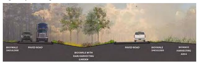
Pushing the travel lanes out to the far edges of the right of way provide space for a wide bioswale for rain harvesting. This image is of Independence Parkway in Houston, Texas, and was prepared for the Texas Land and Water Forum's Low Impact Development Competition. Image courtesy AECOM.
