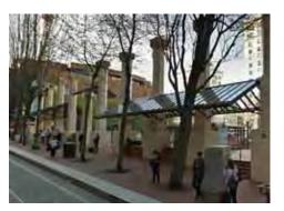
Pioneer Square in Portland, Oregon uses limestone curbs and brick paving to create a safe, attractive pedestrian corridor along the streets. Metal and glass structures provide shelter from bad weather, kiosks provide wayfinding information, and the large columns define the edge of a public space used for events. Image courtesy James Sipes.
