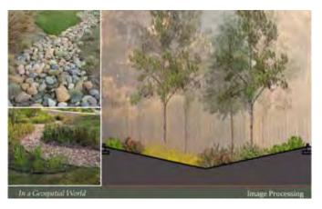
The Texas Land and Water Forum conducted a Low Impact Development (LID) competition in 2009 to explore how LID could be implemented in Harris County. The winning entry for Independence Parkway pushed the roadways to the edge of the right-of-way and created a bioswale in the median. This bioswale is able to handle all run-off from a 100-year storm and it also reduces sedimentation and pollution runoff, and significantly improves aesthetics. Image courtesy AECOM.
