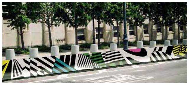
The use of bold, angular geometric forms painted on jersey barriers helps blur the barrier's edges and soften the visual impact. This approach is intended to induce nearby traffic to slow down, producing a safer, more bike- and pedestrian-friendly thruway. Image courtesy John Locke.
