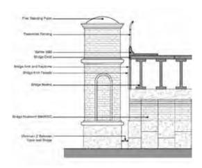
Elevation of a pylon for a Monroe Parkway bridge. Image courtesy EDAW.
