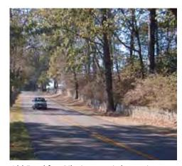
Old Frankfort Pike is a scenic byway in Lexington, Kentucky. The dry stack stone walls, also called 'slave walls,' that line both sides of much of the road were created in the early 1800s from limestone collected in neighboring fields. Dry stone is a building method by which structures are constructed from stones without any mortar to bind them together. Image courtesy A. Crane.
