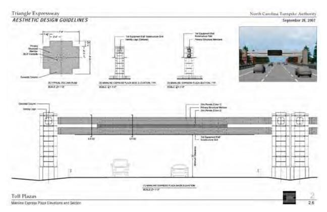
These drawings show the overall layout and details used to construct sign toll gantries and support posts for the Triangle Expressway in Raleigh, North Carolina. The enhanced visual quality of the gantries and supports is consistent with that provided for bridges, noise walls, and other details along the Triangle Expressway. Image courtesy NCDOT.
