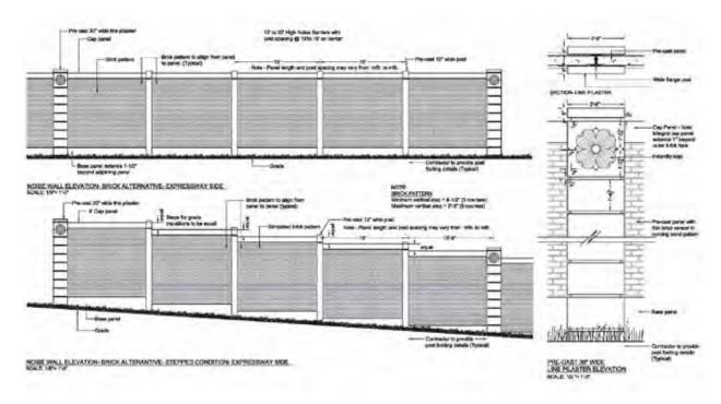
These elevations show the level of detail to be implemented as part the the noise walls used for the Triangle Expressway in Raleigh, North Carolina. The top elevation shows a noise well along level ground, while the bottom elevation shows how the walls would step down to follow the grade for steeper slopes. Image courtesy NCDOT.
