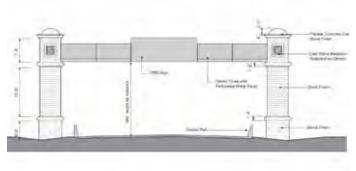
This drawing shows details for a toll gantry and informational signage for the Monroe Parkway. The design elements for the gantries were consistent in design with other parts of the Parkway. Image courtesy EDAW.
