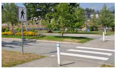
This crosswalk includes stripes in the roadway, bollards to protect pedestrians, and signage to delineate the walks. Image courtesy DepositPhotos.com.
