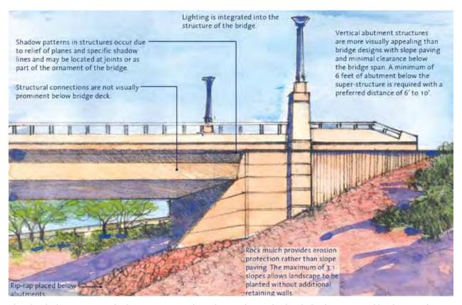
This sketch shows concepts for how to integrate the railings, columns, bridge deck, abutment, and landscaping for a bridge over I-15 in Las Vegas, Nevada. The sketch shows the use of shadow patterns, integrated lighting, vertical abutments structures, rock mulch and rip-rap, and structural connections. Image courtesy NVDOT.
