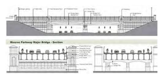
Elevation of a major bridge for the Monroe Parkway. A central pier is used to support the bridge. Image courtesy EDAW.
