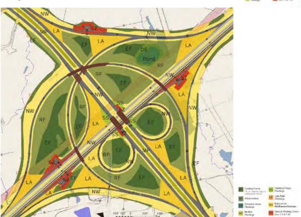
This plan outlines the basic aesthetic guidelines for planting along a four-way interchange that is part of the Triangle Expressway. This serves as a design template for all similar interchanges that are part of the project. Image courtesy NCDOT.
