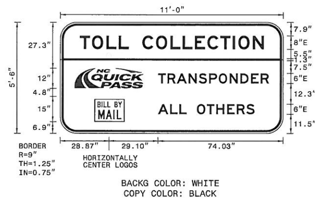
RAMP TOLL GANTRY SIGN PANELS
